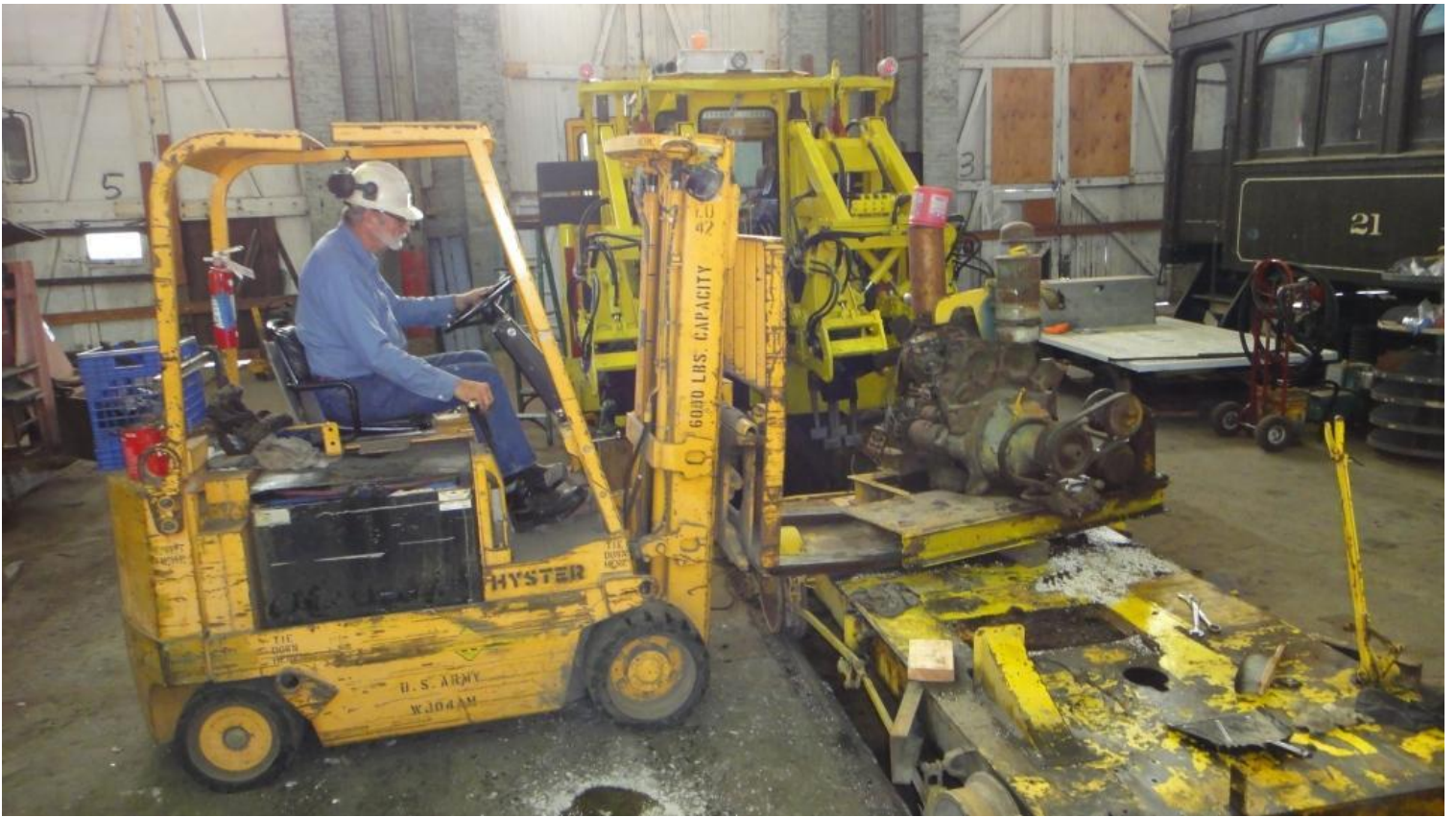
Next, the old GM Diesel is removed
