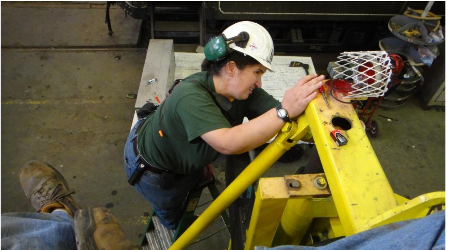
Heather rewiring the front-end red-lights of the J3K Tamper. Notice the nice protective cage that Cliff made.
